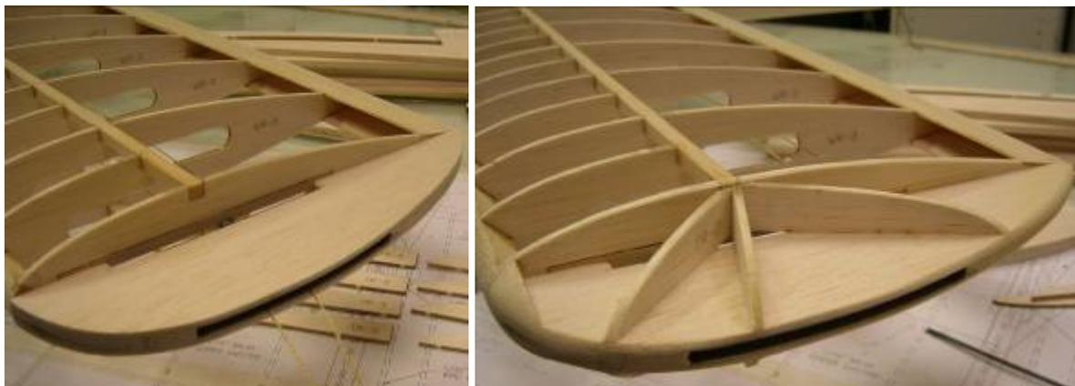
Once done, repeat the process for the outboard wingtip. The adjustable weight box is mounted to the back side of the spars, Install a piece of scrap sheeting between or on the back of the spars so the adjustable weight box has something to hold onto other than the rib. See plans for A.W.B. location.
