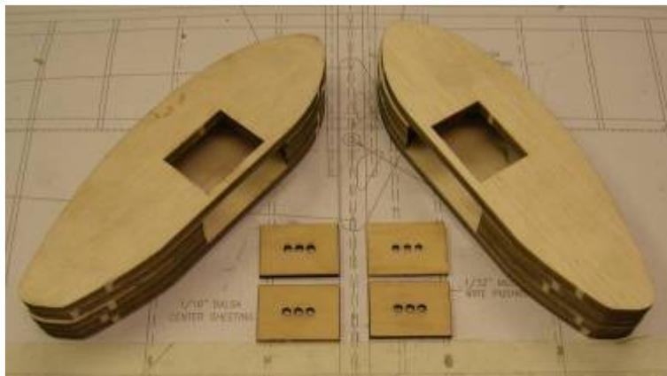
Wheel pant assembly will vary from wheel to wheel, so use these photos as a guide to assembling the wheel pants with the wheels you have chosen for your Spacewalker, once assembled, sand to shape.
