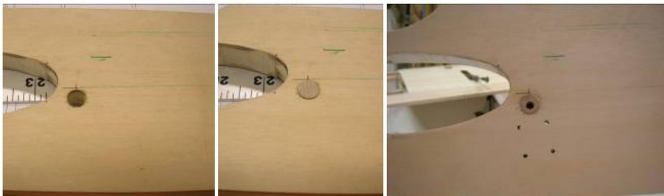
Mount the gear, tank and engine, once mounted mark both sides of the fuselage doublers by tracing around where these objects are mounted. Once done, duplicate these markings to the balsa triplers and relieve balsa triplers as required. See photos.
