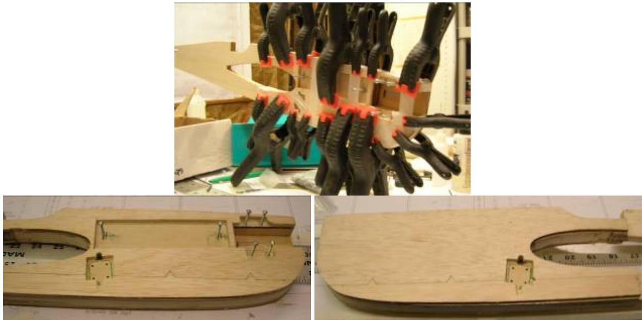
Drill hole for tail wheel wire then epoxy tail wheel block into fuselage, once cured test fit and secure wire.
