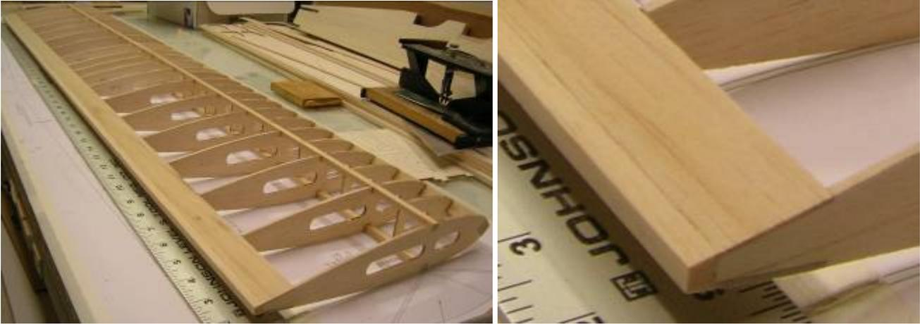
Once done, permanently install the top bellcrank mount (*top one only*) to the rib and spar. Next, carefully remove the wing from your work surface, and then remove the wing rib building tabs from each rib and repeat the process of sanding the T.E. flush with the sheeting.
