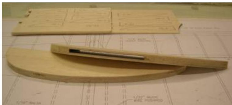
Masking sure you have proper clearance for the leadouts, install the assembled inboard wingtip, tip ribs and scrap balsa L.E. filler on to the wing.
