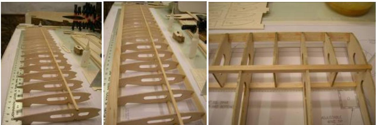
Once done, carefully scarf cut and join the two T.E. sticks together. Always use a long straight edge when joining sticks and sheeting together. Once done, glue the trailing edge on.
