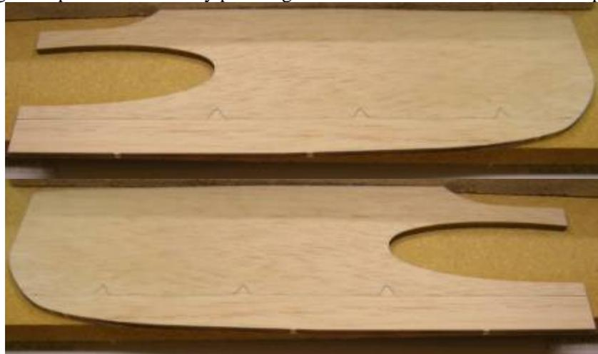
Once done, mark on the fuselage which sides are to receive the glue, this will prevent you from gluing the wrong side.
